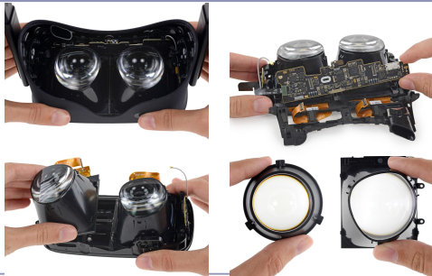
Teardown of an Oculus Rift CV1 showing details of lenses and displays https://www.ifixit.com/Teardown/OculusRiftCV1+Teardown/60612
