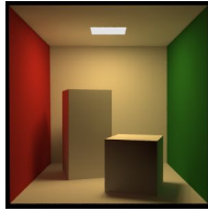
The Cornell Box is a test for rendering software, developed at Cornell University in 1984 by Don Greenberg. An actual box is built and photographed; an identical scene is then rendered in software and the two images are compared.
